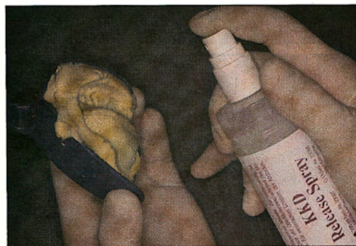
Fig. 3 Surface tension of silicone reduced with KKD Release Spray.
